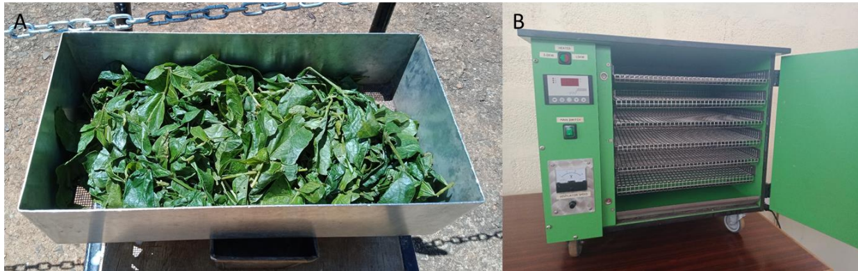
Figure 12: Other techniques of dehydration of cowpea leaves. A-Sun-drying of blanched cowpea leaves, B- Forced air ventilation oven drier
